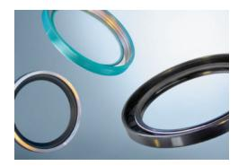
Radial shaft seals are used to seal rotating shafts. The seal works radially and is fixed inside the housing bore by means of a retaining ring, and at the same time seals statically. The dynamic sealing lip works radially against the rotating shaft.
