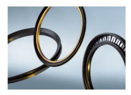
Axial shaft seals are used to seal rotating shafts. The low-friction and wear-resistant seals work axially and are usually mounted securely on the shaft, i.e. the seals rotate with the shaft.
